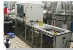
制备膜电极的连续超声喷涂设备。 Ultrasonic spraying machine for the continuous CCM production.
