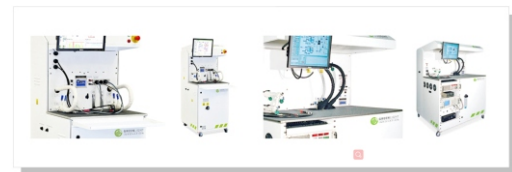
小面积膜电极性能评价测试工作站(左)和大面积膜电极寿命测试工作中(右)。 Small-area single-cell testing station (activity, upper) and large-area single-cell testing station (longevity).
